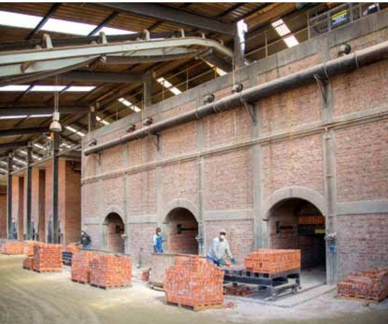
»5 The VSBK kiln at Langkloof Bricks, an energy-efficiency improvement project facilitated by the EECB Project, uses 82.5 g of coal per kg of fired brick. Just 2.5 g of this is external fuel during the firing process
