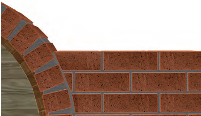
15.9 - The wooden support is removed and a portion of the uncompleted brickwork on the one side is shown.
